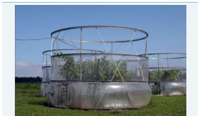
Figure 1: Open-top chambers placed over Chambourcin and Vidal grapevines allowing exposure of vines to ambient and 63% ambient ozone concentrations.
